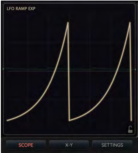
Traveler Scope showing LFO waveshape
